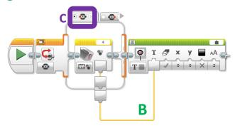
C. Different options in the switch can connect to the same wire
