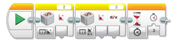
By reading the angle of the gryo then the rate+angle the gyro sensor gets recalibrated. Make sure to run these blocks when the robot is still.
