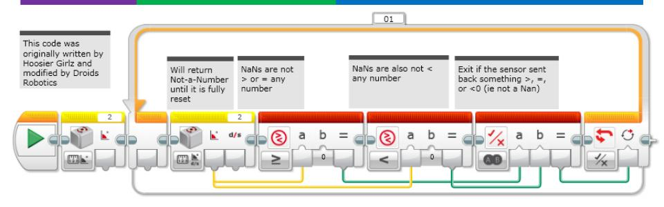
This version of the calibration leaves the gyro in rate+angle mode. This is useful if you use the rate output.
