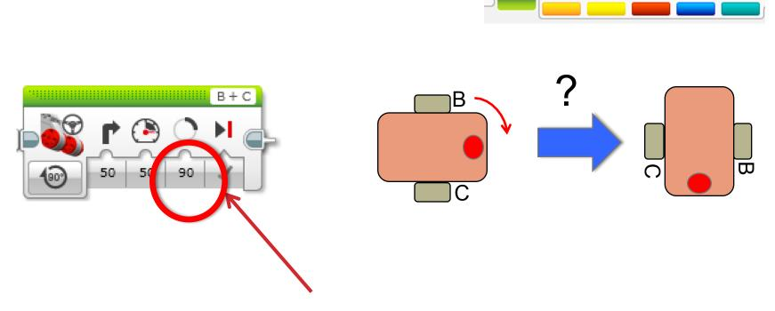
Program your robot to turn 90 degrees....Does the robot actually turn 90 degrees if you just pick 90 degrees for distance? Ans. NO! Solution on next page
