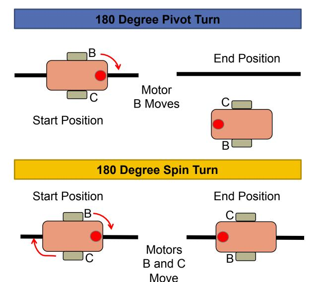
Notice where the robot ends in both pictures after a 180 degree turn.
